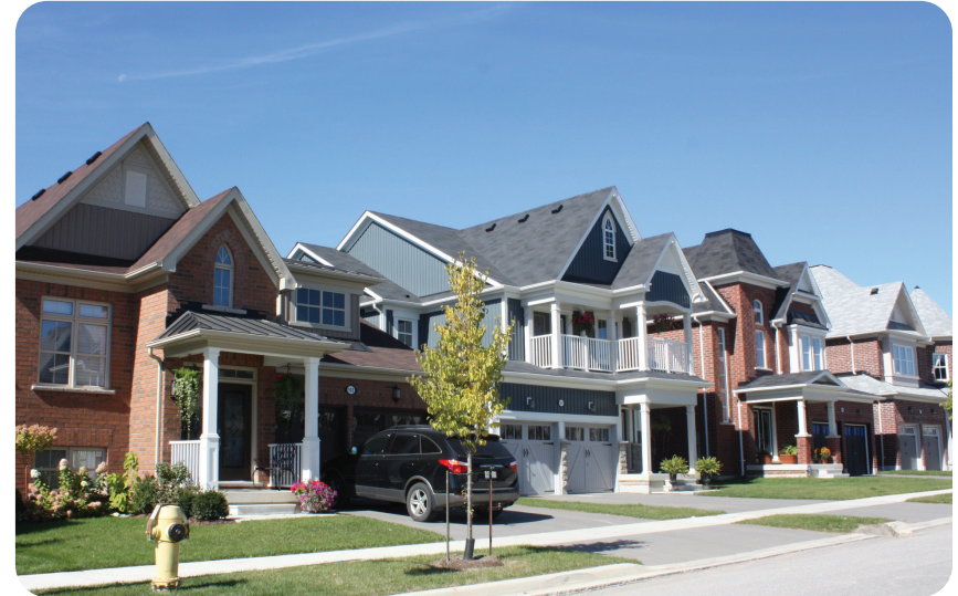
Variety of façade elements (porches, walls, bays) that extend in front of the garage assist with articulation and animation of the streetscape
