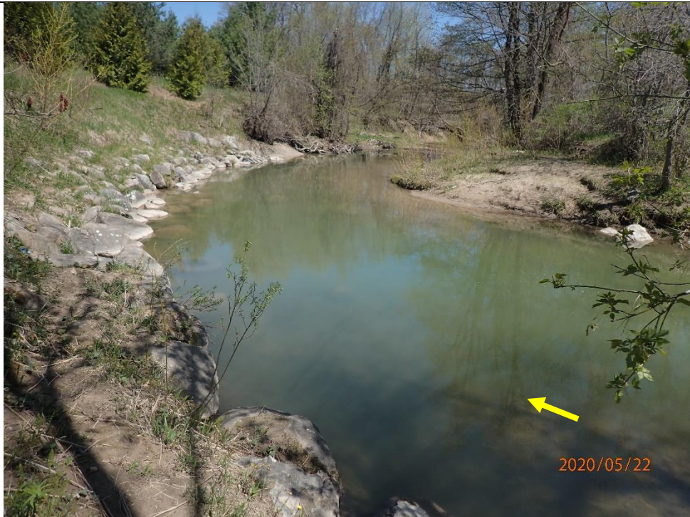
Riffle/pool sequencing was good throughout the reach. Pools had an average depth of approximately 1.5 m. Siltation was identified within the pools indicating aggradation within the channel.
