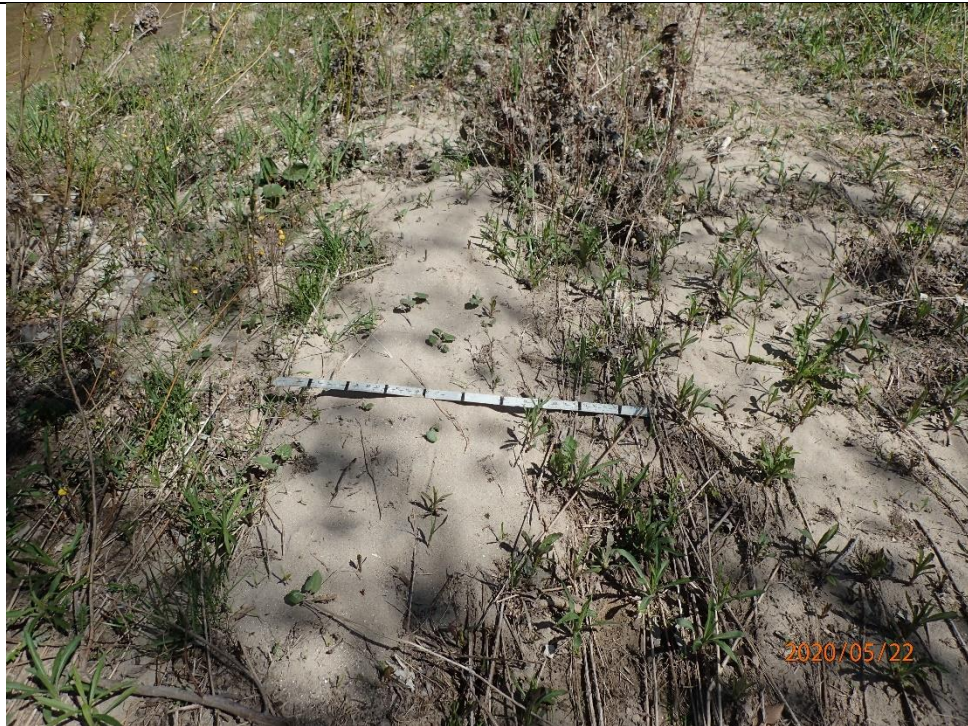
Photograph taken of a fresh large sand deposit along the top of low banks. Deposition in the overbank zones was common within the reach providing evidence of aggradation.
